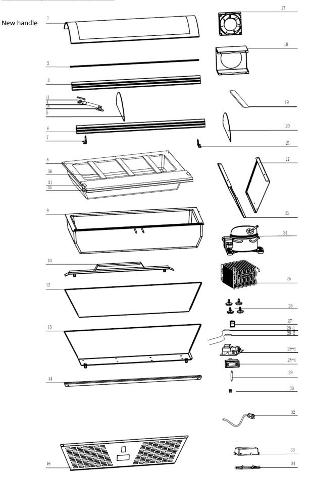
Exploded diagram and spare parts list GL178 Rev.7
